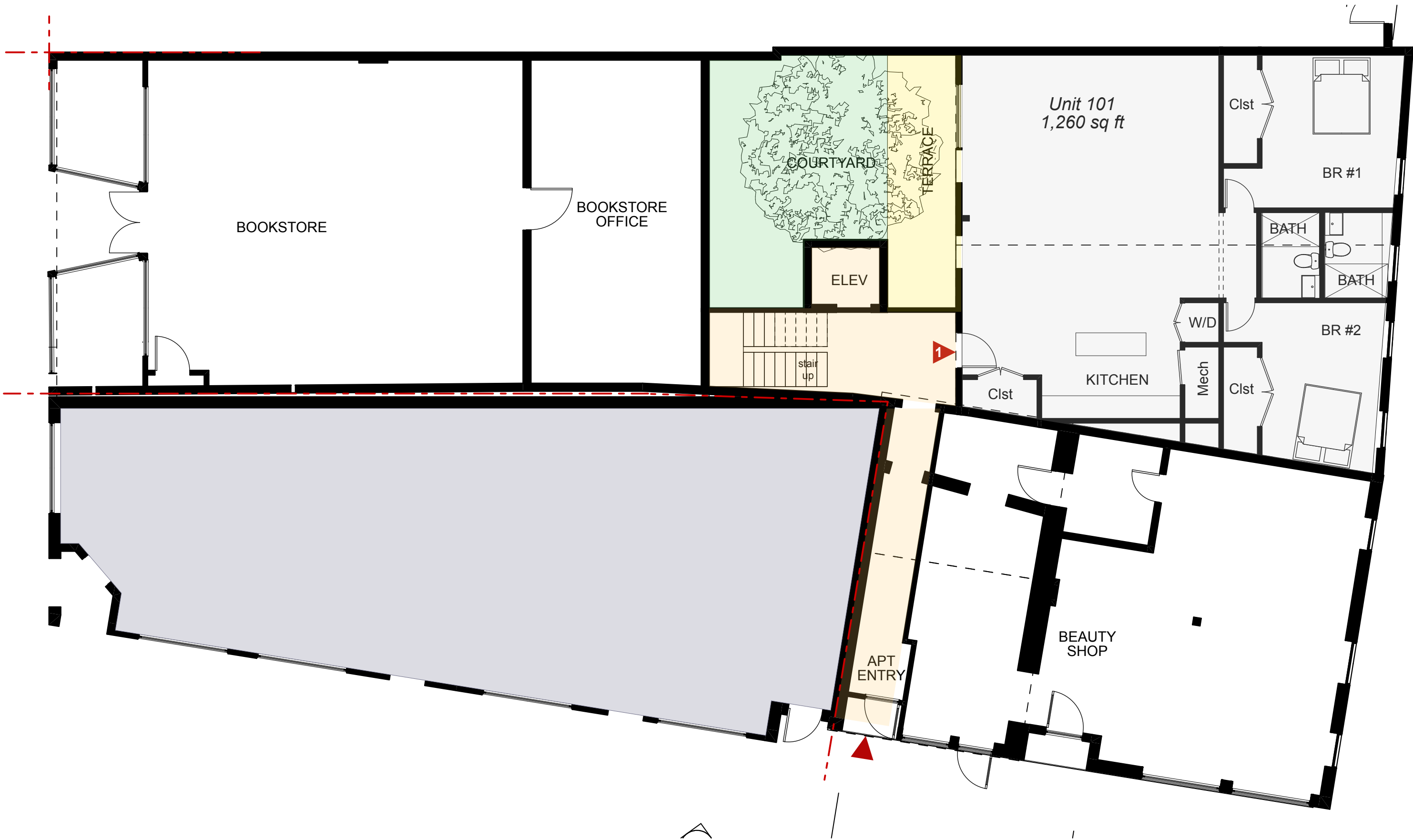
1 Proposed 1st Floor Plan SCALE: 1/8" = 1'-0"
