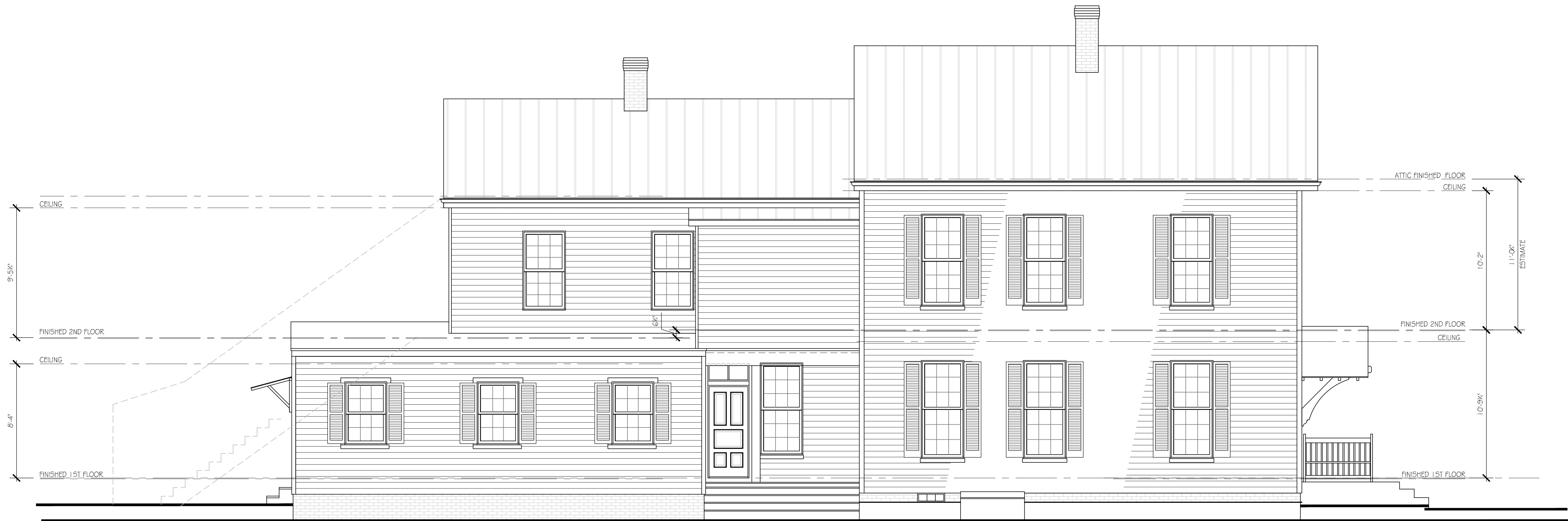
EAST ELEVATION - Existing SCALE: 1/4" = 1'-0"
