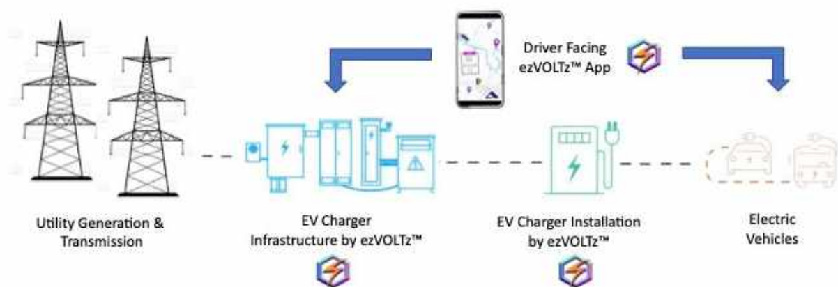
Fig. 2. ezVOLTz™ Services in the EV Charging Value Chain
