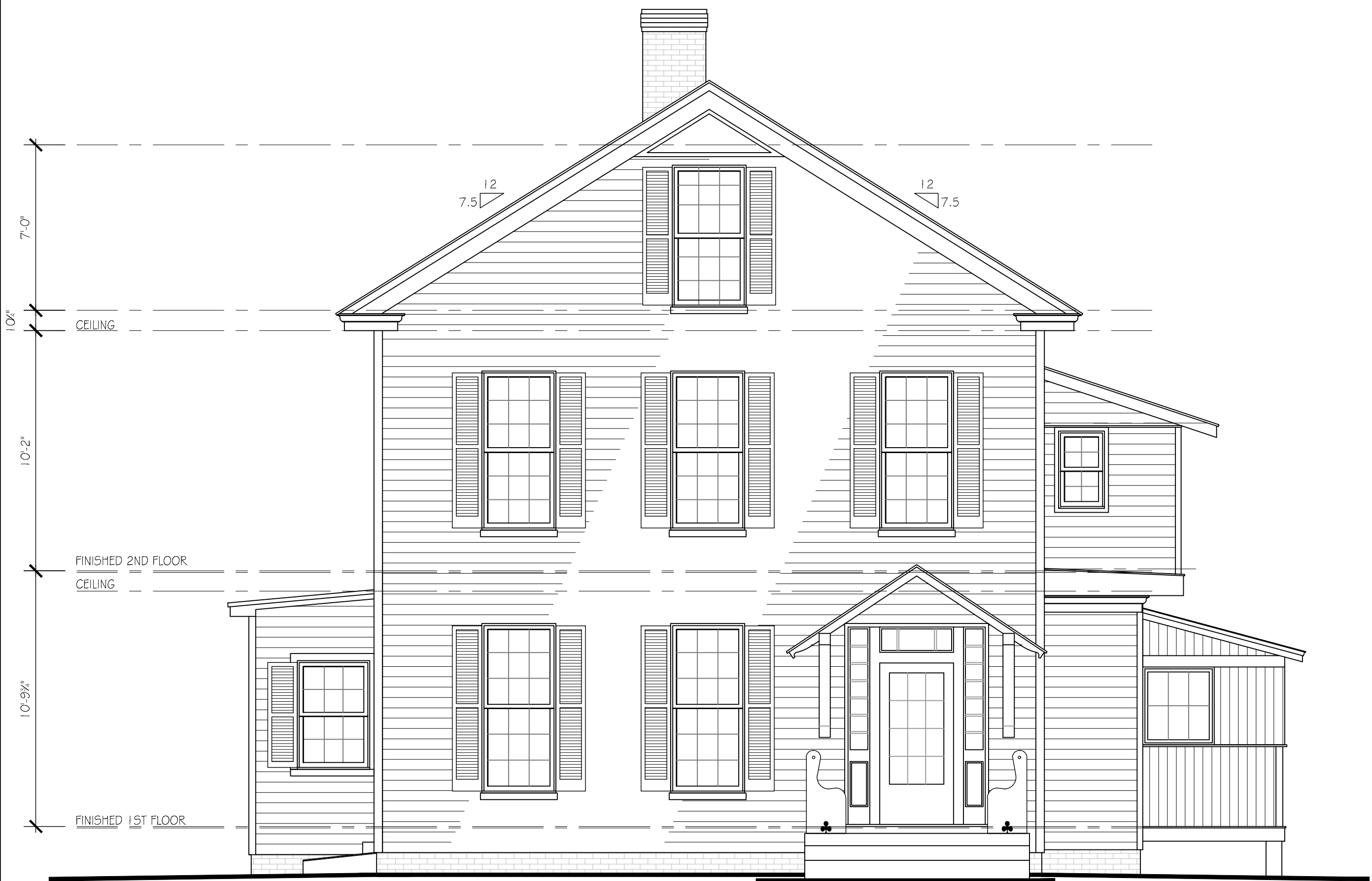
NORTH ELEVATION - Existing SCALE: 1/4" = 1'-0"
