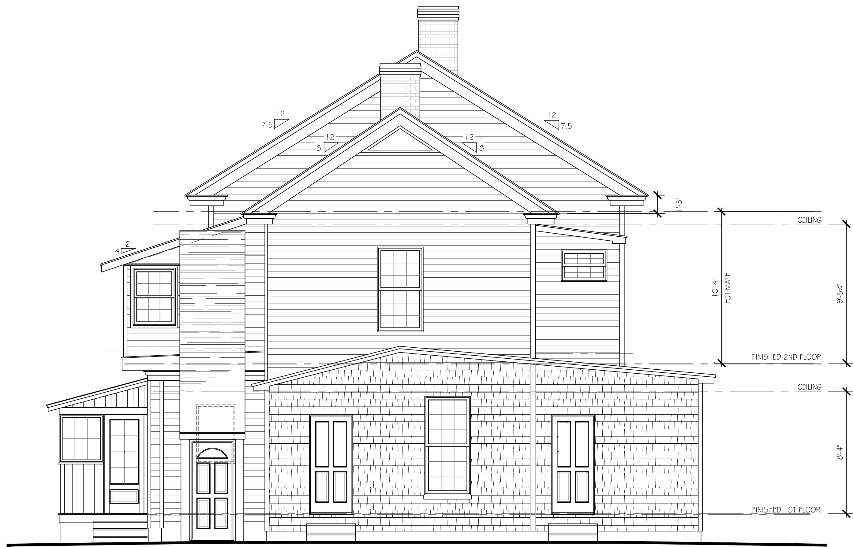
SOUTH ELEVATION - Existing SCALE: 1/4" = 1'-0"
