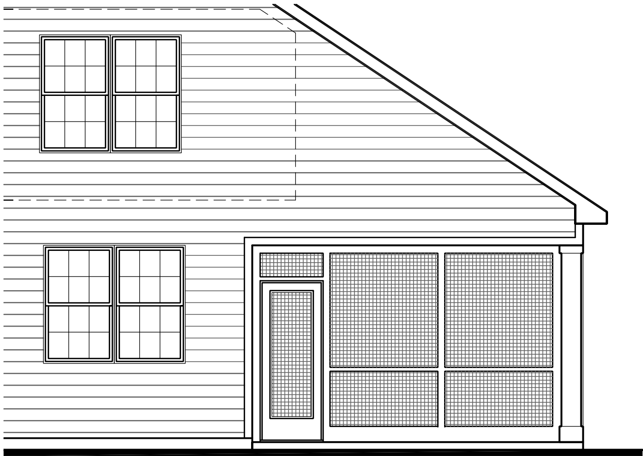
Partial Rear Elevation w/ Opt Screened Porch
