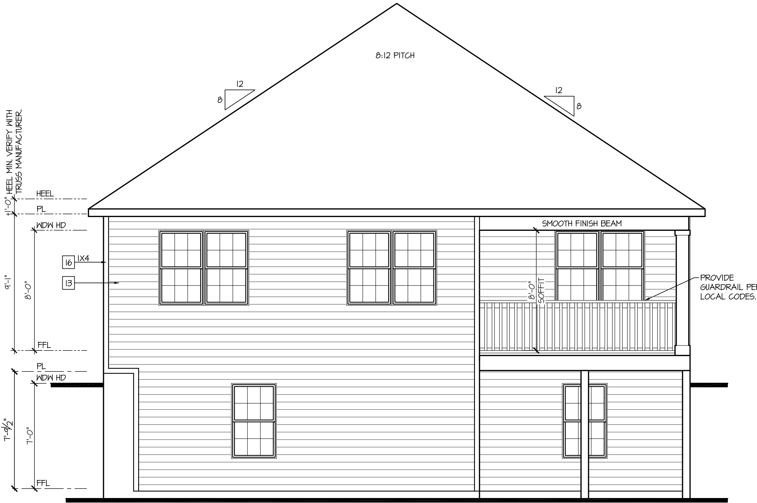
Rear Elevation w/ Opt Walk-Out Basement
