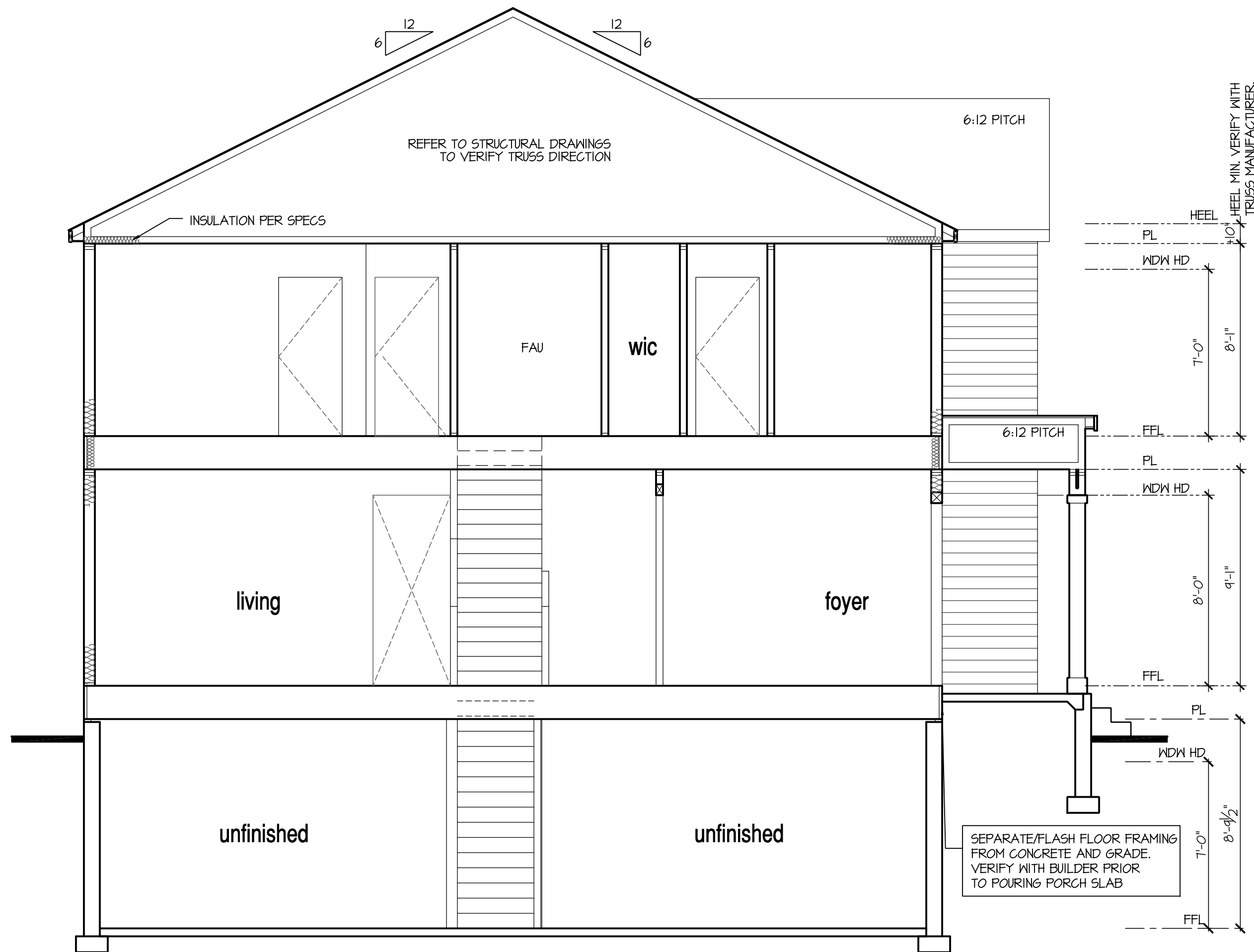
Building Section 1 at Opt 9' Basement
