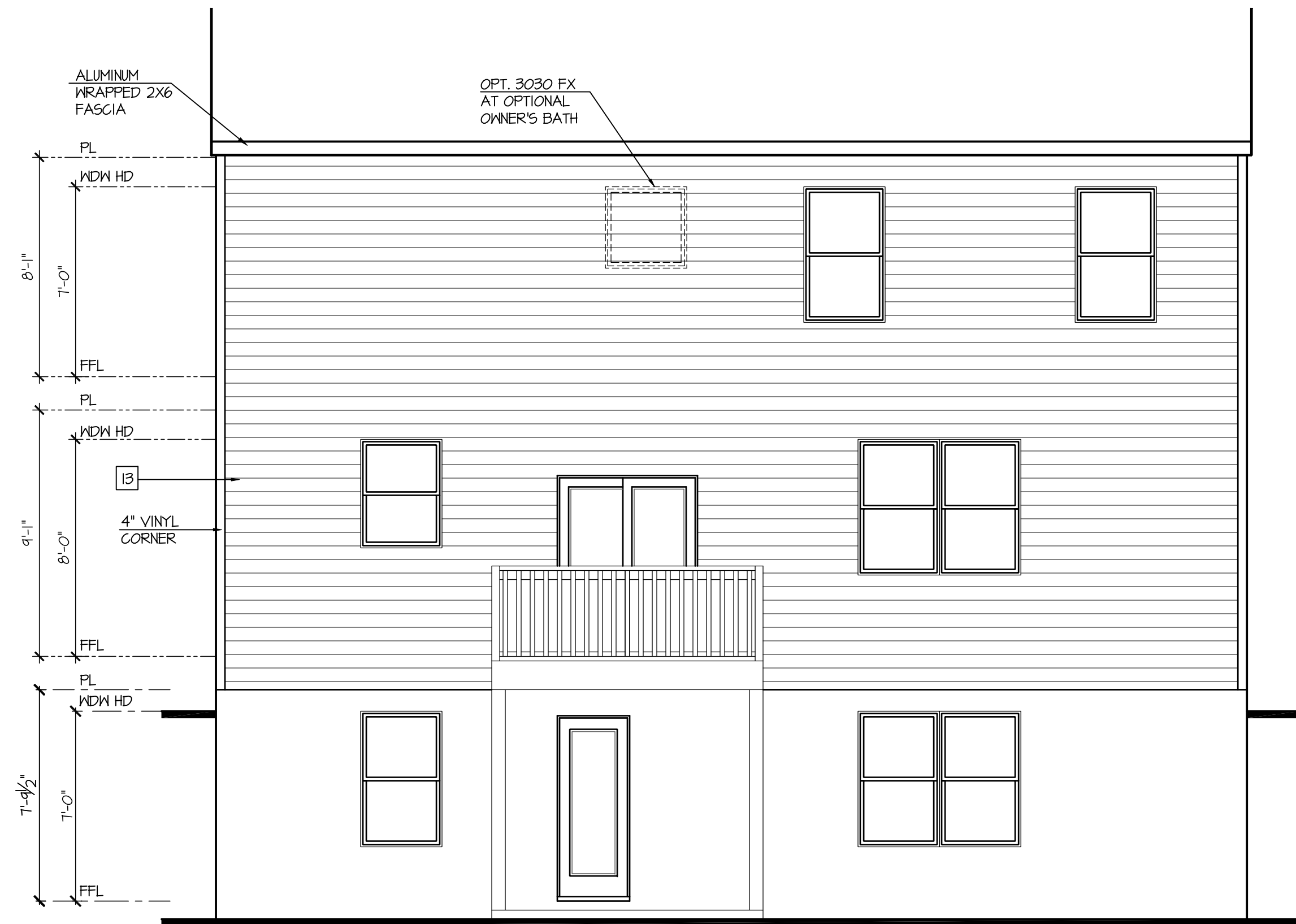
Partial Rear Elevation w/ Opt Walk-Out Basement
