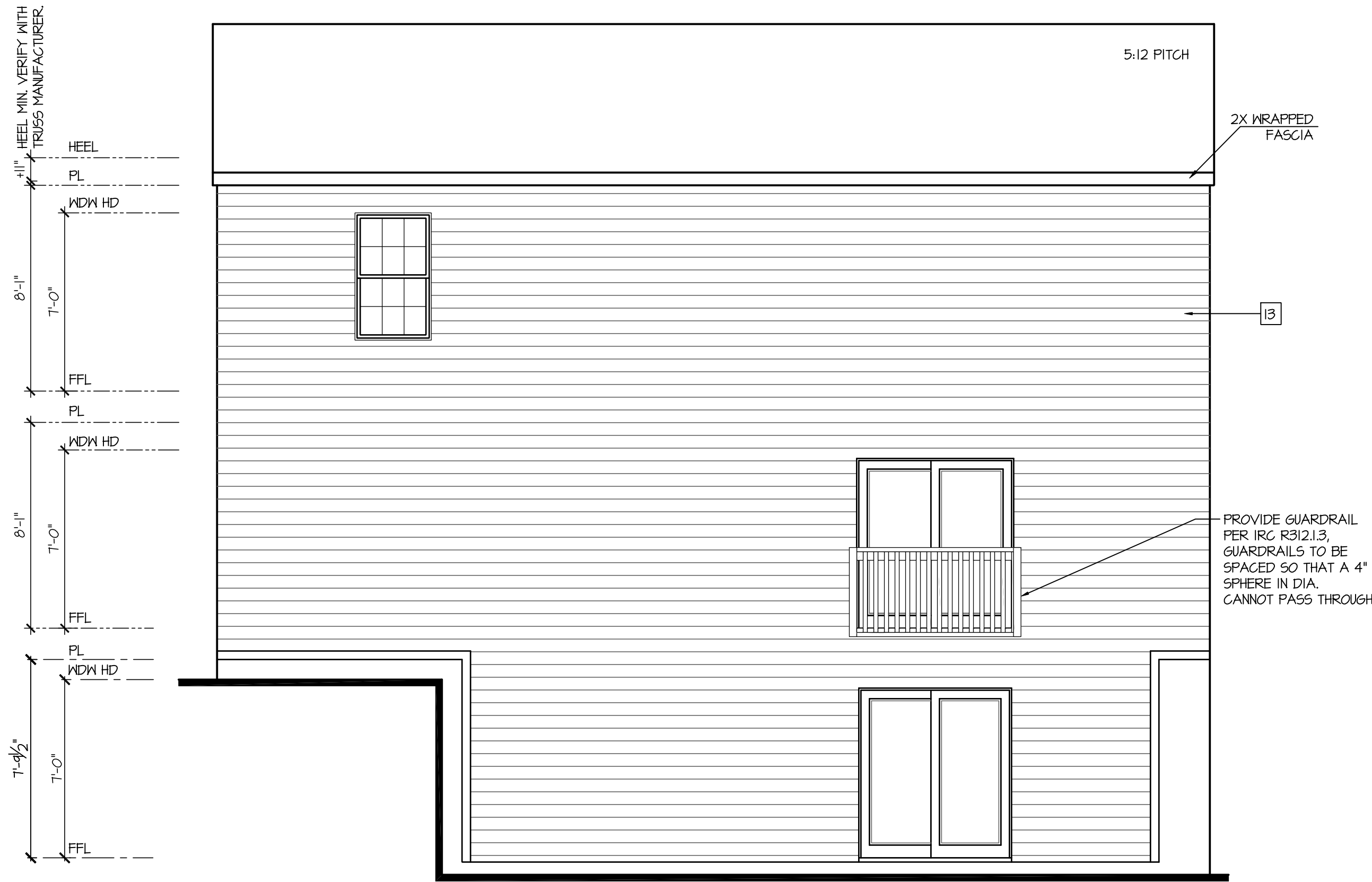
Rear Elevation w/ Opt Walk-Out Basement
