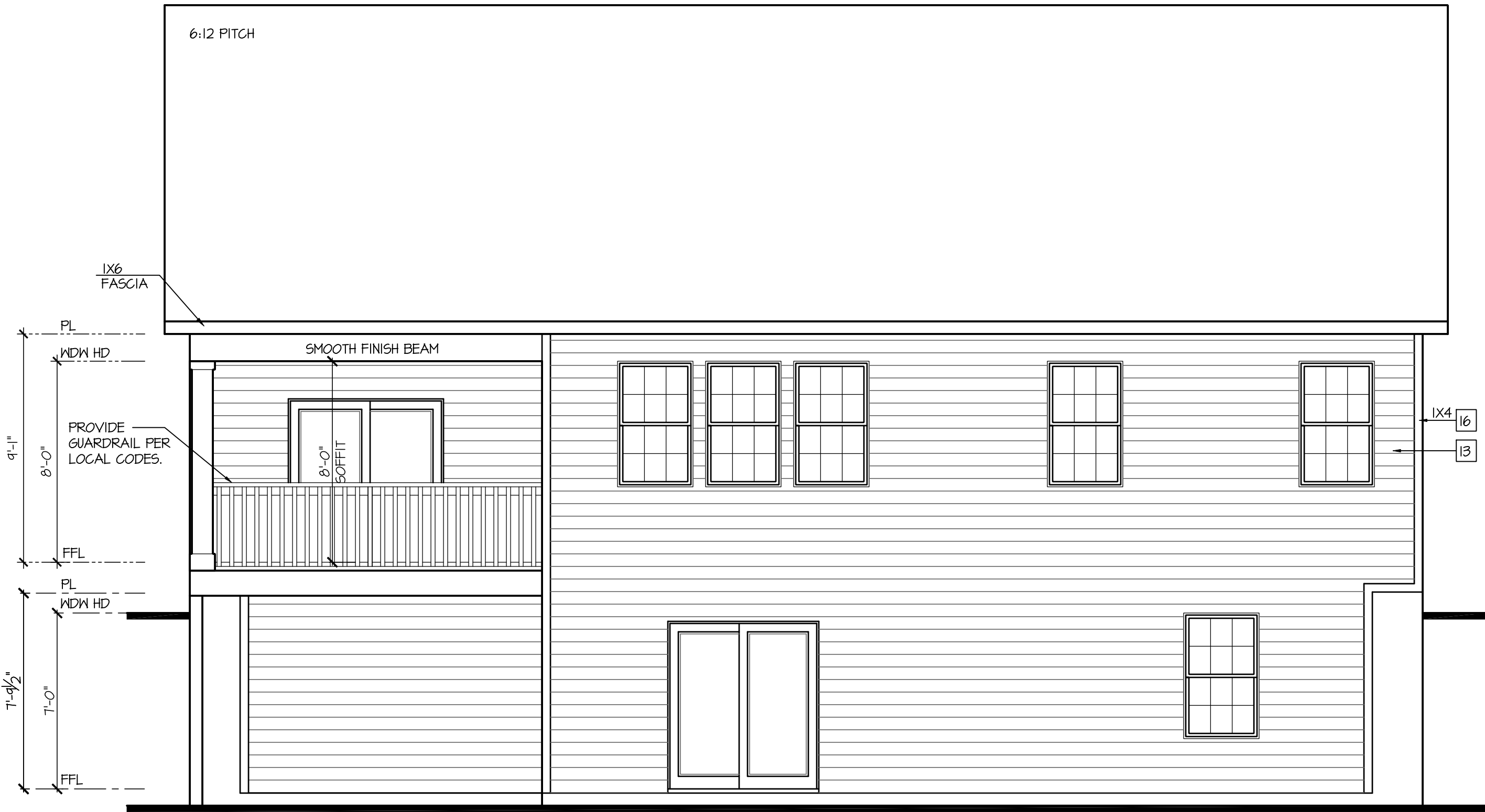
Rear Elevation w/ Opt Walk-Out Basement
