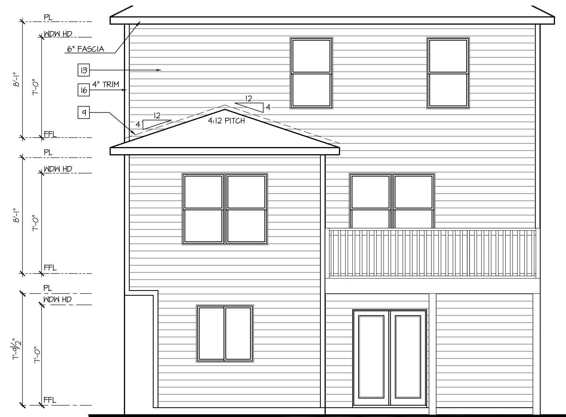
Rear Elevation w/ Opt Walk-Out Basement
