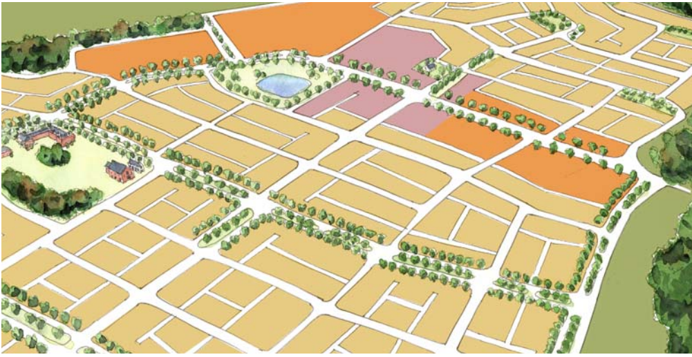
Blocks with Lot Types ■ High-Density Residential Lots ■ Civic, Institutional, and Park Land ■ Medium-Density Residential Lots ■ Mixed-Use Lots
