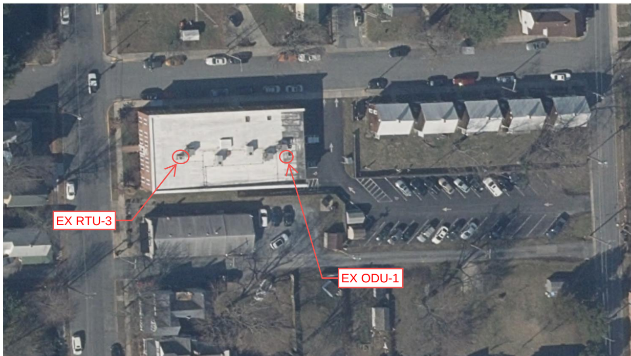
Satellite view – HVAC units to be replaced
