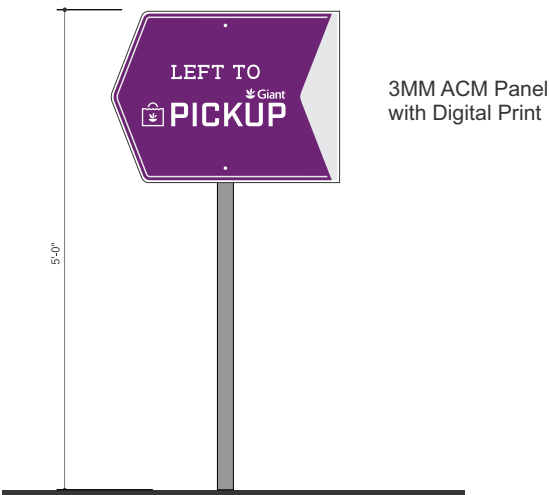
1 D/F POST & PANEL SIGN FACE REPLACEMENT SCALE: 1/2" = 1' - 0"
