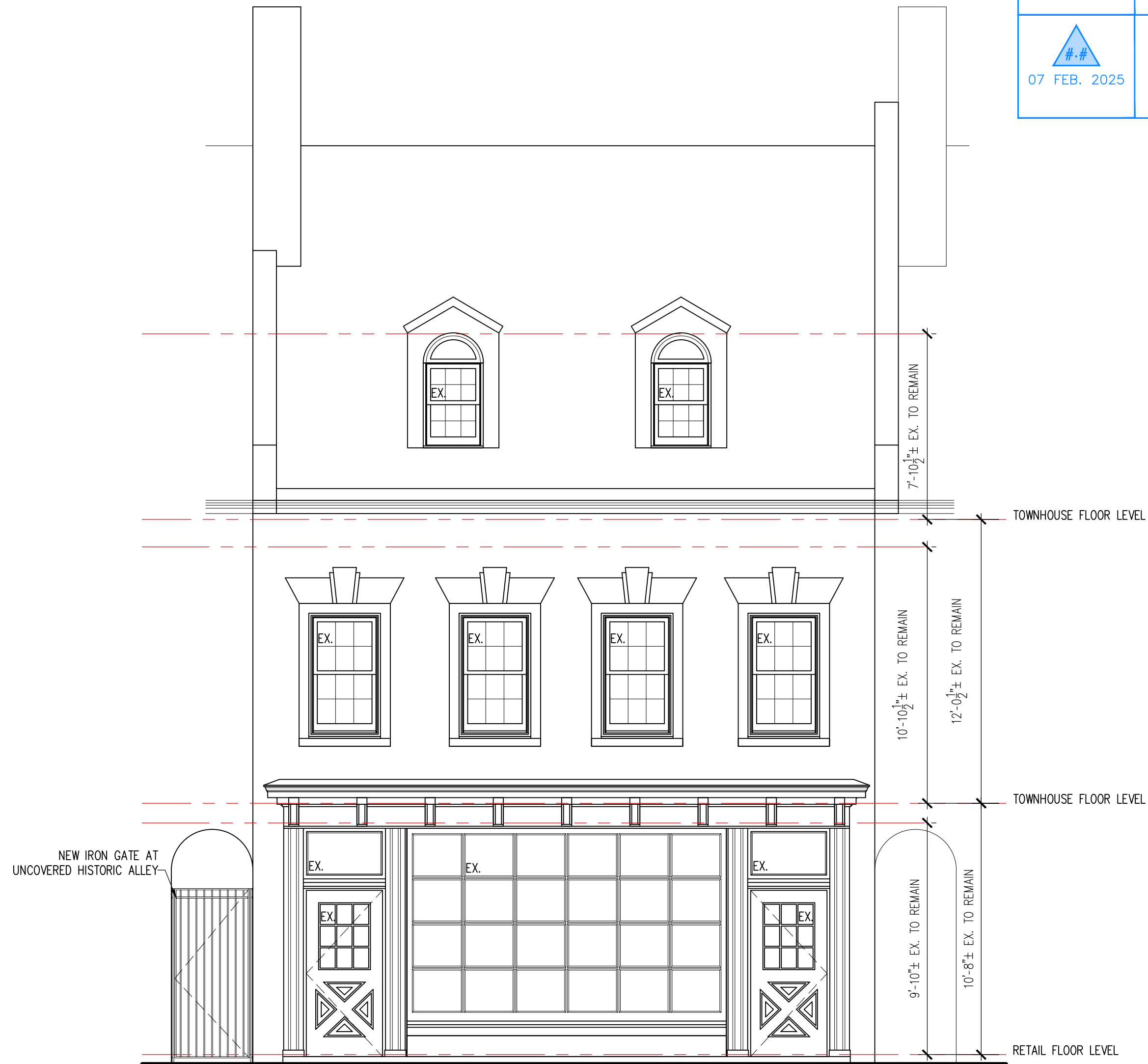
4 FRONT (EAST) ELEVATION 1/4"=1'-0"
