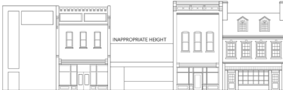
INAPPROPRIATE FACADE ARRANGEMENT INTERRUPTS STREET RHYTHM
