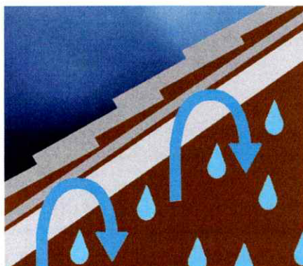
Typical synthetics "Non-breathable" synthetic underlayments can trap harmful moisture.
