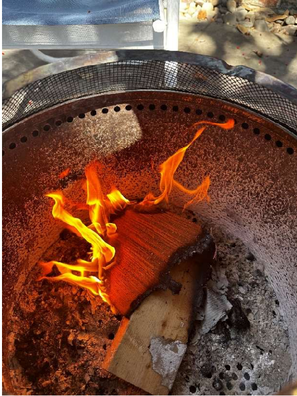
Figure 11: Cedar roofing material structurally consumed by fire within minutes of ignition.
