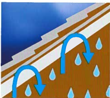
Typical "non-breathable" synthetic underlayments can trap harmful moisture
